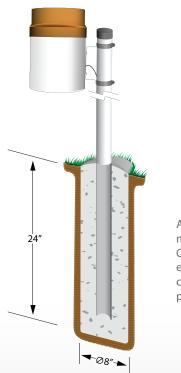
At left is a TE525 mounted onto a CM310 pole that is embedded directly in a concrete pad (-NP no pedestal base option).
