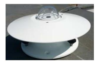
A pyranometer is used to measure the total energy from the sun. When leveled in the horizontal plane, this is called the Global Shortwave Irradiance (GLOBAL) and when positioned in a plane of a PV Array, it is called the Total Irradiance in the Plane of Array (TPA). Inverted, a pyranometer is used to measure the Reflected or Albedo Irradiance (ALBEDO). A pyranometer can also be shaded from the direct beam of the sun to measure the Diffuse Shortwave Irradiance (DIFFUSE).
