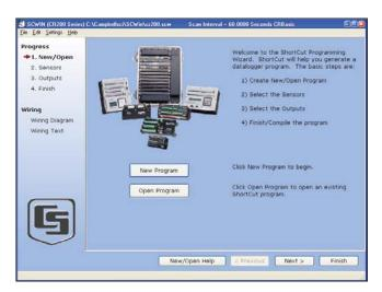
Short Cut provides a wizard-like interface for generating datalogger programs.
