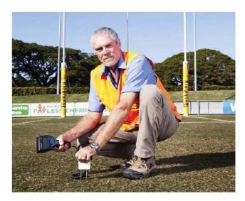
The Hydrosense II is a portable, handheld device for easily obtaining soil measurements. It is the next generation of the Hydrosense soil-water measurement system. Improvements over its predecessor include a more rugged probe design, additional navigation buttons for the display, expanded memory, an internal GPS receiver, Bluetooth communications, and more powerful PC software.
