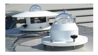
A pyranometer is used to measure the total energy from the sun. When leveled in the horizontal plane, this is called the Global Shortwave Irradiance (GLOBAL) and when positioned in a plane of a PV Array, it is called the Total Irradiance in the Plane of Array (TPA). Inverted, a pyranometer is used to measure the Reflected or Albedo Irradiance (ALBEDO). A pyranometer can also be shaded from the direct beam of the sun to measure the Diffuse Shortwave Irradiance (DIFFUSE).
