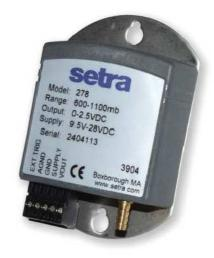
The CS100 includes a switching circuit that allows the datalogger to power the barometer only during measurement, which reduces power consumption. Sensor warm-up and measurement time are one second minimum.
