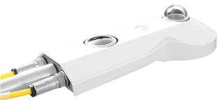
CNR 4 is a four-component net radiometer for accurate and reliable measurements and can be used as the reference instrument for a network of lower performance net radiometers. There are four separate signal outputs and the integrated temperature sensors can be used to calculate the FIR radiation. The screw-in mounting rod, bubble level, and cables with waterproof connectors, make installation easy. The white sun shield reduces solar heating of the instrument body.
