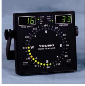
Wind direction information is clearly displayed on a circular compass pattern of LEDs. Multicolored segments give a quick visual indication of current direction and direction variability. Front panel brightness control allows adjustment for best viewing in any light.
